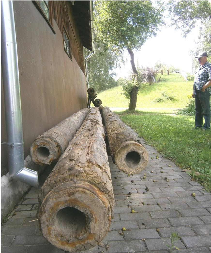
**Figure 1.** The water pipes of water-supply system in Jelgava
